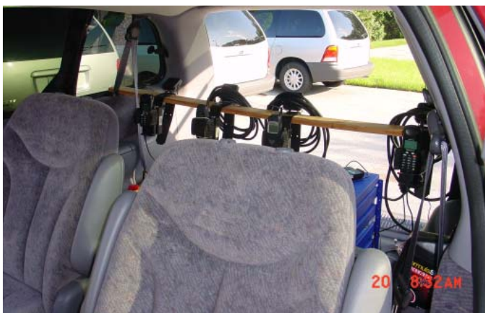
Figure 1. Rear test rack with phones installed.
